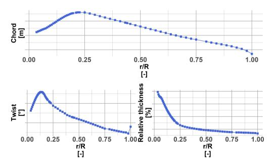
Figure 2. The scanned blade geometry: chord, twist and relative thickness distribution against the normalised radius.
