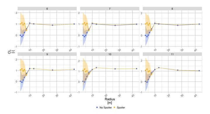
Figure 11. The blue square ( $\blacksquare$ ) shows the  $C_L$  evolution along the blade radius without spoiler, the orange dot ( $\blacksquare$ ) shows the  $C_L$  evolution along the blade radius with spoiler. Each subplot shows the results for a wind speed (m/s) whose value is given in the title.
