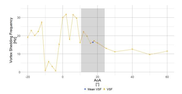
Figure 17. Plot of the angle of attack versus the Vortex Shedding Frequency for the "spoiler" case radial position R6 ( $\frac{r}{R} = 13.3\%$ ) calculated in 2D CFD. The blue square ( $\blacksquare$ ) shows the mean VSF (interpolated VSF at the mean angle of attack of the time series), the orange dots ( $\bullet$ ) show evolution of the VSF depending on the angle of attack. The shaded area shows the standard deviation of the angle of attack time series.
