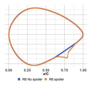
Figure 1. Overimposed aerofoil shapes at radial position R6 ( $\frac{r}{R} = 13\%$ ): the blue square ( $\blacksquare$ ) shows the no spoiler coordinates while the grange dot ( $\blacksquare$ ) shows the spoiler coordinates
