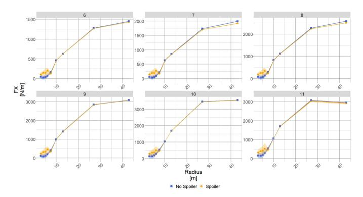
Figure 13. The blue square ( $\bigcirc$ ) shows the force normal to the rotor plane evolution along the blade radius without spoiler, the orange dot ( $\bigcirc$ ) shows the normal force to the rotor plane evolution along the blade radius with spoiler. Each subplot shows the results for a wind speed (m/s) whose value is given in the title.
