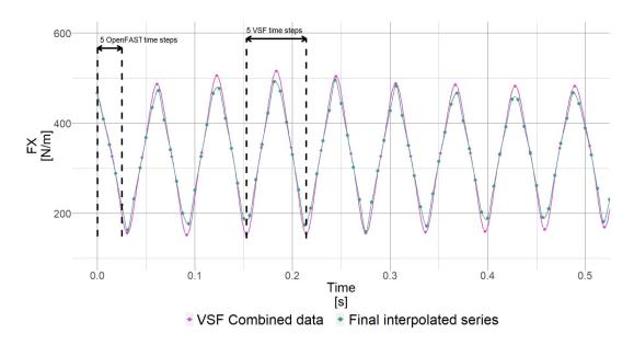
Figure 21. Generation of the final time series using the sampling rate from OpenFAST ( $\Delta t_{OF} = 0.0063$ s).
