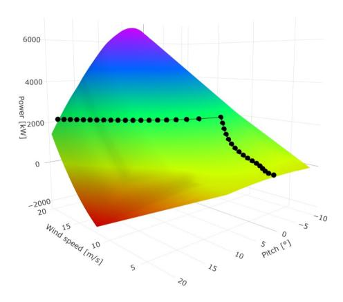
Figure 9. Power surface response with varying pitch settings for different wind speed. Each coloured dotted lines represents a wind speed. The black stars (\*) represent the pitch settings for maximum power production the spoiler case using mean aerodynamic polar. The horizontal black dashed dotted line is the turbine's rated optimal pitch settings for maximum power generation.
