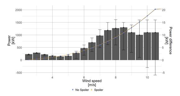
Figure 15. Power curve close-up for the low wind speeds. The blue square (■) shows the power curve without spoiler, the orange dot ●) shows the power curve with spoiler. The black bars show the difference between the mean "spoiler" and mean "no spoiler" case.
