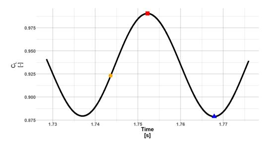
Figure 3. "Spoiler" case  $C_L$  evolution in time  $\alpha = 6^{\circ}$  and  $Re_c = 3 \times 10^6$ . The blue triangle ( $\blacktriangle$ ) corresponds to the minimum  $C_L$ , the red square ( $\blacksquare$ ) corresponds to the maximum  $C_L$ , the orange dot ( $\bullet$ ) corresponds to the mean  $C_L$ .
