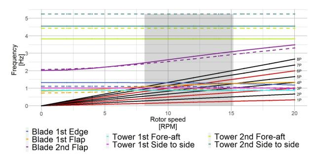
**Figure 4.** Campbell diagram comparison between the NREL reference turbine and the ENGIE Green scaled one. The solid lines shows the NREL response and the dashed lines the ENGIE Green turbine's response. The dark shaded area illustrates the ENGIE Green's turbine range of operation.
