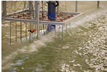
Figure 10: Breaking wave impact at a monopile from model tests of the DeRisk project (Source: Bredmose et al., 2016)
