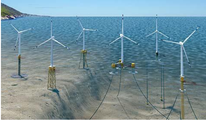
Figure 9: At water depths up to 60 m, offshore wind turbines can be installed on fixed-bottom foundations. Deeper than approximately 60 m, floating substructures are needed. (Image credit Josh Bauer, NREL)
