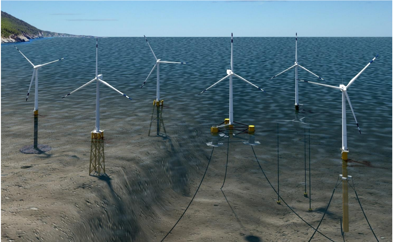
1410 Figure 9: At water depths up to 60 m, offshore wind turbines can be installed on fixed-bottom foundations. Deeper than approximately 60 m, floating substructures are needed. (Image credit Josh Bauer, NREL)
