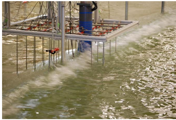
1515 Figure 10: Breaking wave impact at a monopile from model tests of the DeRisk project (Source: Bredmose et al., 2016)
