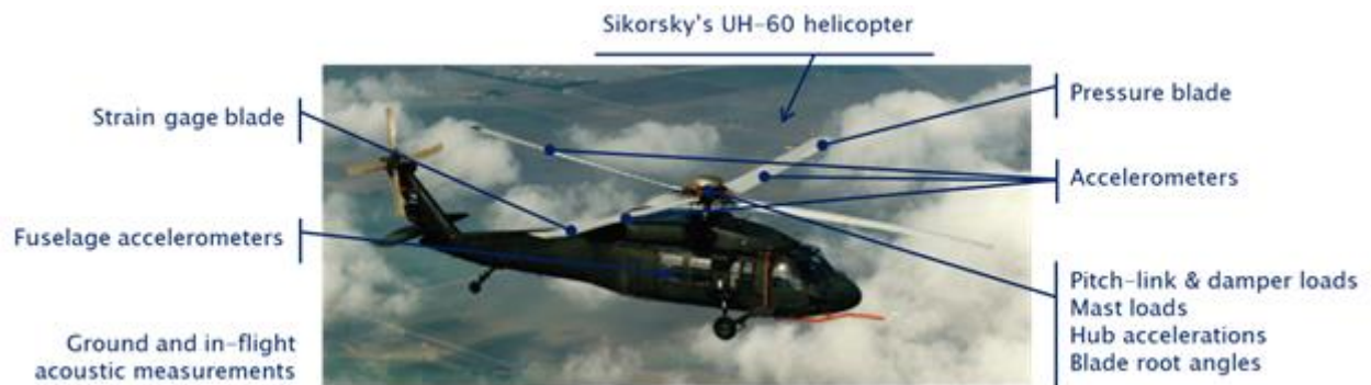
Figure 7: A highly instrumented UH-60A flying over the San Joaquin Valley in California during the UH-60A Airloads Flight Test Program. The data set collected in these experiments led to major advances in the modeling and simulation of rotorcraft vehicles. Wind energy science needs similar high-quality, fully open-access data sets, which are indispensable for validating the models and tools that will enable the design of the wind turbines of the future. (Photo from https://rotorcraft.arc.nasa.gov/Research/Programs/uh_60_program.html )
