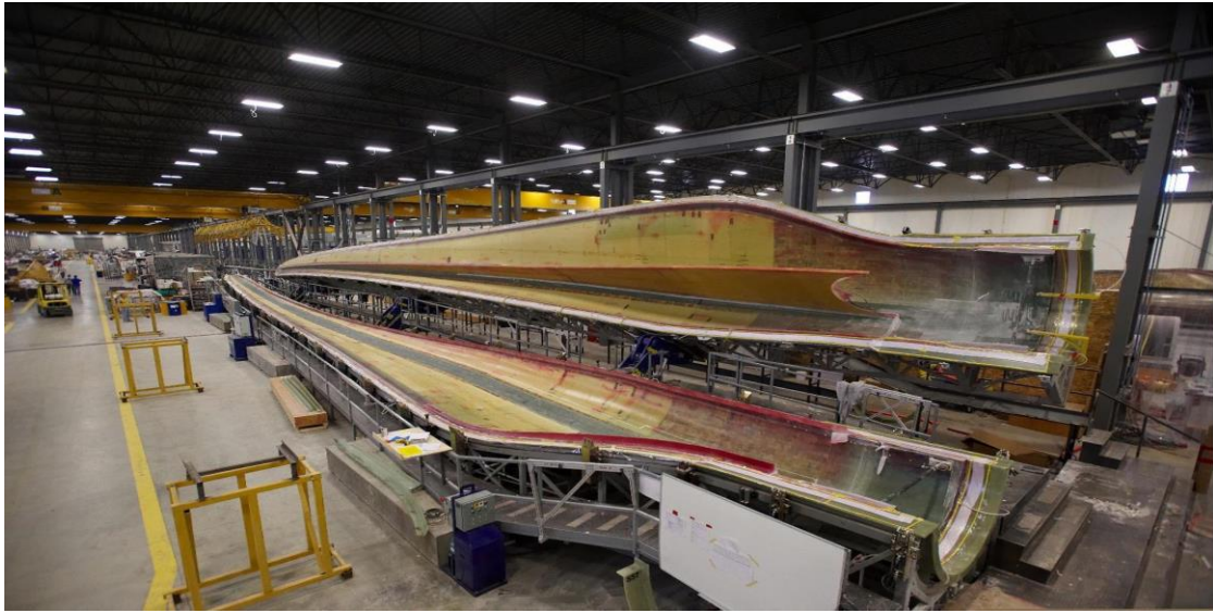
1715 Figure 14: A 40 m wind turbine blade in production demonstrating the size and complexity of manufacturing wind turbine blades at modern scales. The assembled blade skins and internal webs are about to be bonded together, a process which has tolerances of 1 mm in some cases, and requires both speed and attention to detail for the adhesive material to bond effectively. (Photo credit TPI Composites)
