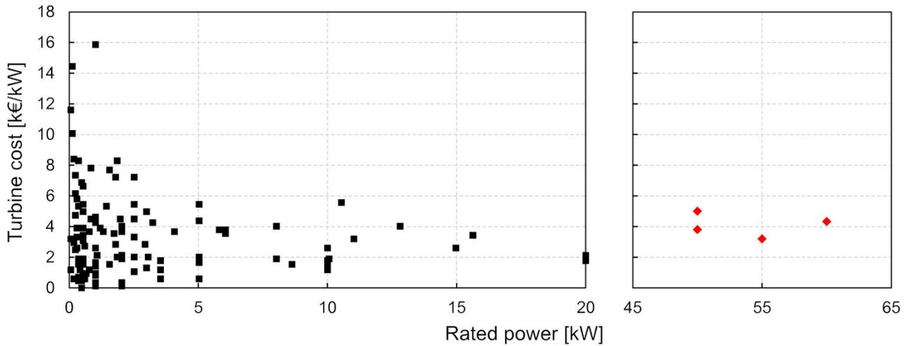
195 **Figure 5 - Turbine purchase cost survey for rated power lower than 20 kW (Kaldellis and Zafirakis, 2012) and around 50 kW**
