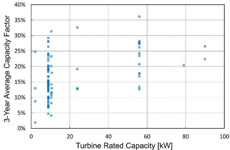
Figure 7 – Three-year average capacity factor for several U.S. wind projects. Data from (Orrell et al., 2020).
