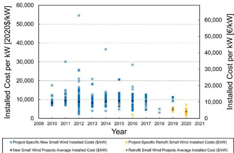
244 **Figure 6 - Installed cost per kW for new installed or retrofit installed projects in the United States (Orrell et al. 2021).**
