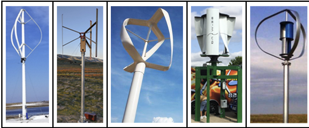
556 Figure 13 - Common VAWT archetypes found in the current DWT market. From left to right: Darrieus Troposkien (photo credit: 557 Chava Wind); H-Darrieus (photo credit: Xflow Energy); H-Darrieus with helix shape (photo credit: PRAMAC); Savonius (photo 558 credit: BE Wind); combined Savonius-Darrieus (photo credit: HiVAWT).
