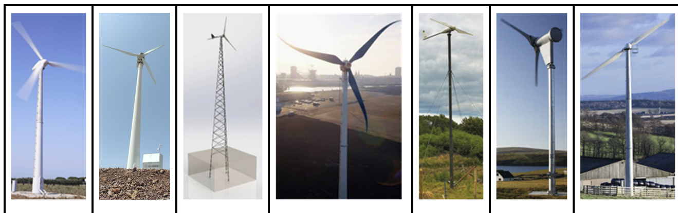
533 Figure 11 - Common HAWT archetypes found in the current DWT market. From left to right: Upwind, active pitch and yaw (photo credit: Tozzi Nord); upwind, stall-controlled and active yaw (photo credit: Eunice); upwind, stall-controlled and tailed passive yaw (photo credit: NREL pix 49511); downwind, stall-controlled, passive yaw (photo credit: Eocycle – formerly XANT); upwind, tailed passive yaw, furling (photo credit: Bornay); downwind, pitch or pitch-coning controlled, passive yaw (photo credit: SD Wind [formerly Proven]); downwind, stall-controlled, passive yaw and teeter (photo credit: Ryse Energy [formerly Gaia]).
