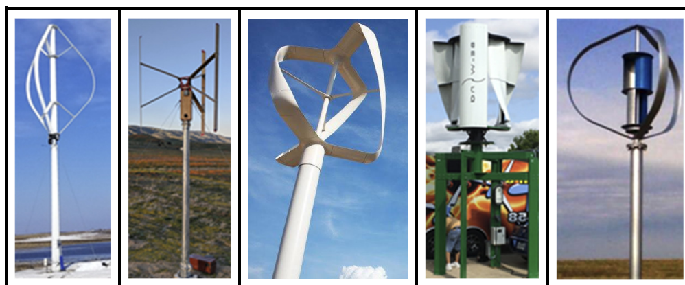
540 Figure 12 - Common VAWT archetypes found in the current DWT market. From left to right: Darrieus Troposkien (photo credit: Chava Wind); H-Darrieus (photo credit: Xflow Energy); H-Darrieus with helix shape (photo credit: PRAMAC); Savonius (photo credit: BE Wind); combined Savonius-Darrieus (photo credit: HiVAWT).
