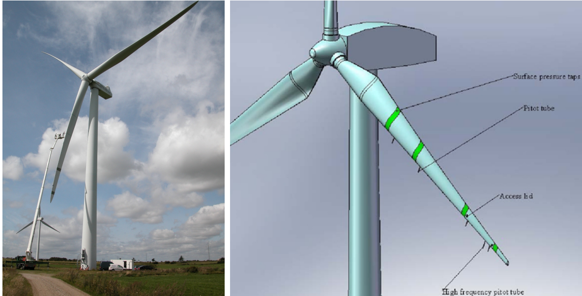
Figure 1. Danaero turbine and instrumentation (Bak et al., 2010)
