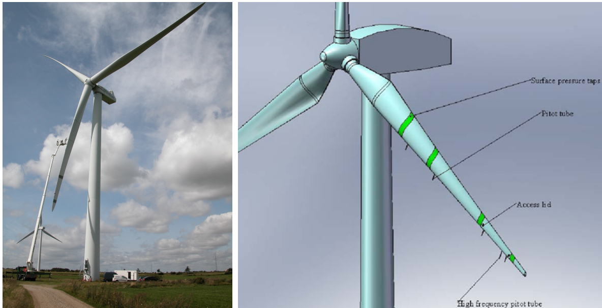
Figure 1. Danaero turbine and instrumentation (Bak et al., 2010)
