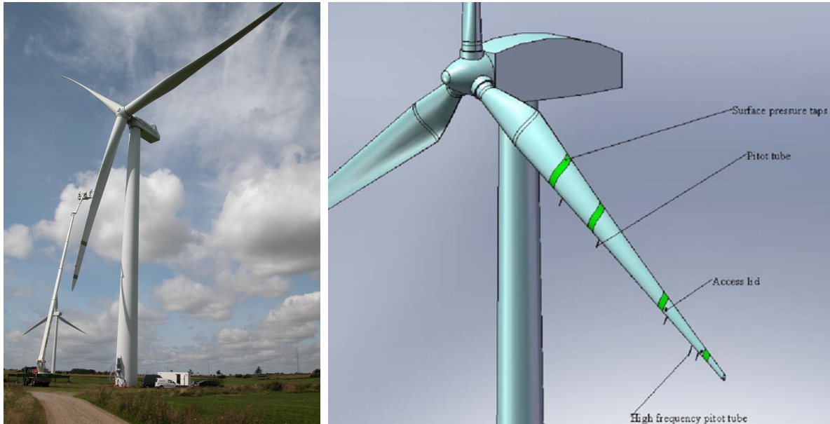
Figure 1. Danaero turbine and instrumentation (Bak et al., 2010)
