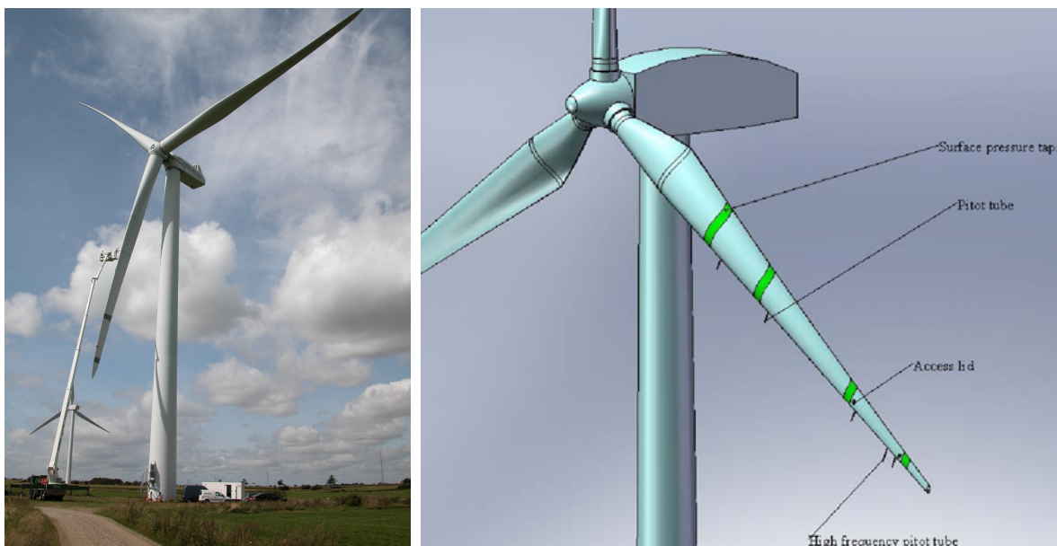
Figure 1. Danaero turbine and instrumentation (Bak et al., 2010)
