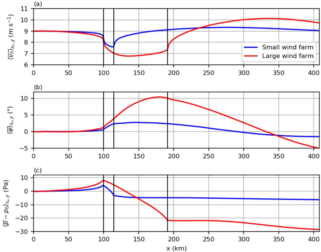
**Figure 3.** Horizontal wind speed (a), wind direction (b) and perturbation pressure (c) along  $x$ . All quantities are averaged along  $y$  and one turbine spacing along  $x$ . Vertical black lines indicate LE and TE of the small and large wind farm.
