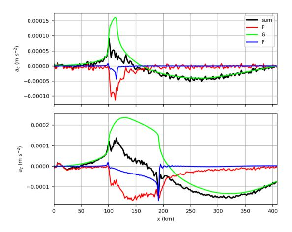
Figure 5. Crosswise forces (perpendicular to streamlines) at hub height along x, averaged along y for the small wind farm (top) and large wind farm (bottom). Shown are the divergence of the vertical turbulent momentum flux (resolved + SGS) F, the geostrophic forcing G (difference between geostrophic pressure gradient force and Coriolis force) and the perturbation pressure gradient force P.
