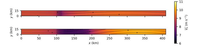
**Figure 2.** Mean horizontal wind speed at hub height for the small wind farm (top) and large wind farm (bottom). Wind direction is indicated by streamlines.
