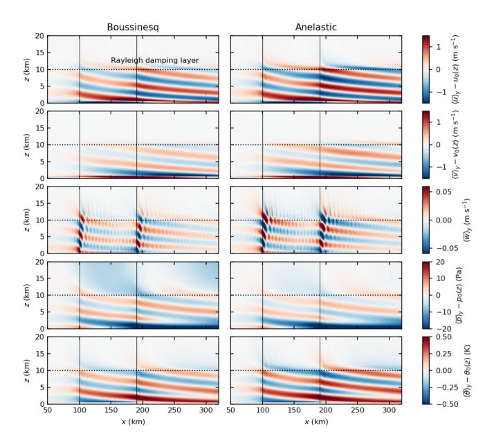
**Figure A1.** Wave fields for the test simulation with Boussinesq approximation (left) and anelastic approximation (right). All quantities are averaged in time and along y and are given as deviations to the inflow profile.
