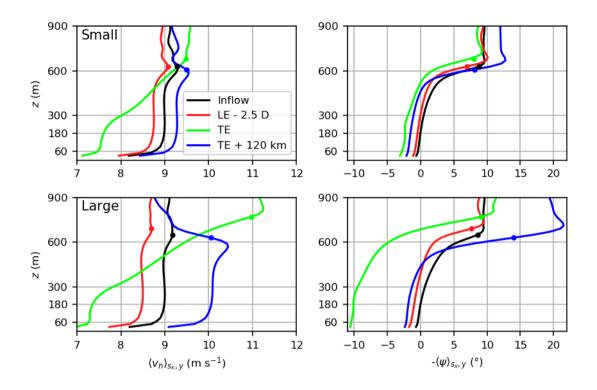
Figure 8. Vertical profiles of the horizontal wind speed (left) and the wind direction (right) for the small wind farm (top) and the large wind farm (bottom). The profiles are averaged in time, along y and over one turbine spacing along x. Horizontal lines are shown at  $z=60\,\mathrm{m}$  (rotor bottom),  $z=180\,\mathrm{m}$  (hub height),  $z=300\,\mathrm{m}$  (rotor top) and  $z=z_i=600\,\mathrm{m}$  (BL height at the inflow). Dots mark the BL height at the respective x-location.
