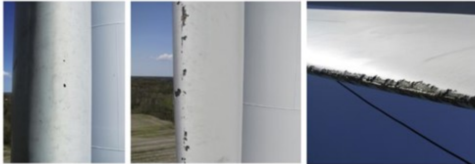
Figure 19. Changes to the LE surface due to impact with a different degree of severity, From left: LEE at an early stage, severely damaged coating and LEE starts to wear the shell material. Adapted from Keegan et al. (2013); Rempel (2012)
