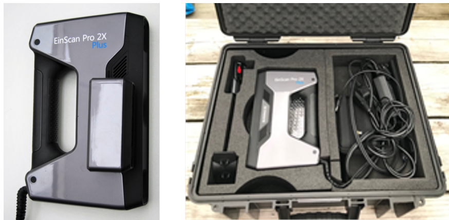
Figure 20. EinScan Pro 2X Plus Handheld 3D Scanner and the flight case with the equipment, photographed by TNO
