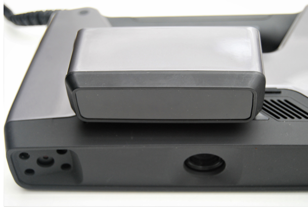
Figure 22. Prima pack add on plugged in the handheld scanner, photographed by TNO
