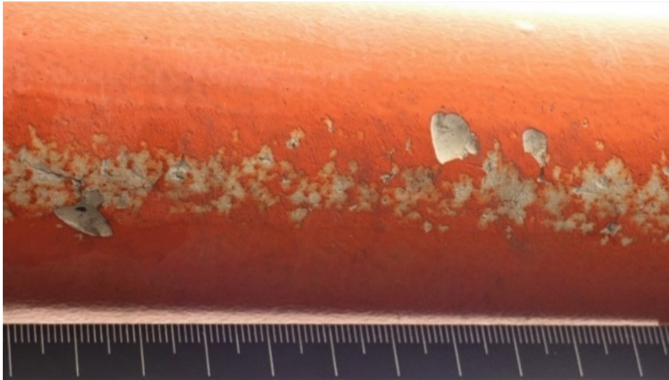
Figure 18. LEE damage on the tip section of a WTB, photographed by TNO
