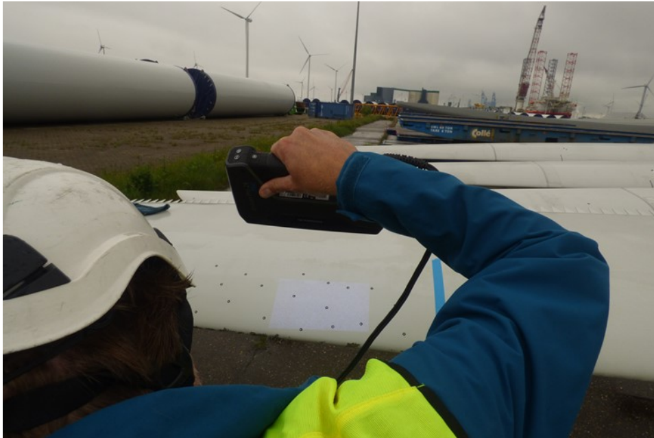
Figure 23. 3D scanning of a tip section of a WTB using sticker markers, photographed by TNO
