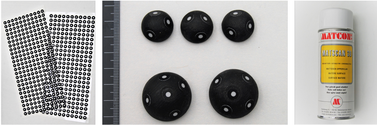
Figure 21. From left to right: 3D marker stickers, large spherical markers, 3D scan anti reflection spray, photographed by TNO
