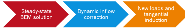
Figure 1. Process of induced velocity correction by the dynamic inflow model. Note that the "steady-state BEM solution" item only refers to the use classical momentum theory and airfoil unsteady effects are included in the evaluation of the instantaneous airfoil coefficients according to the selected model (e.g., Snel, 1997; Hansen et al., 2004).
