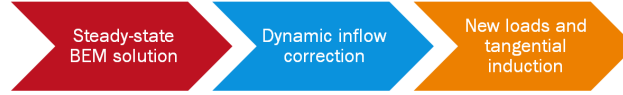
Figure 1. Process of induced velocity correction by the dynamic inflow model. Note that the "steady-state BEM solution" item only refers to the use classical momentum theory and airfoil unsteady effects are included in the evaluation of the instantaneous airfoil coefficients according to the selected model (e.g., Snel, 1997; Hansen et al., 2004).
