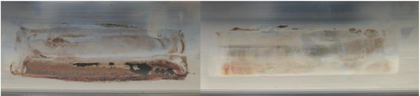
225 **Figure 8:** Two wear marks with 2.5° amplitude; left: tested with 5°/s (ID III), right: tested with 0.8°/s (ID IV)
