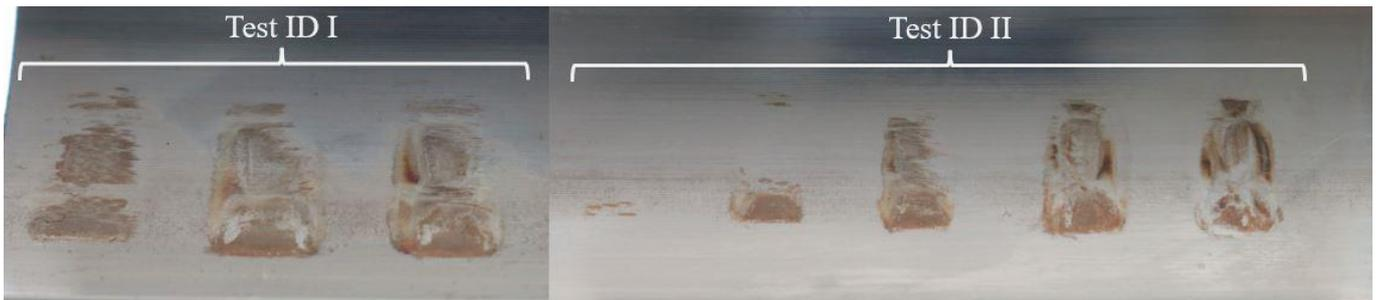
205 **Figure 6: Three wear marks obtained with contact pressures of 2.5 GPa in test ID I (left), five wear marks obtained with contact pressures of 2.0 GPa Test ID II (right)**
