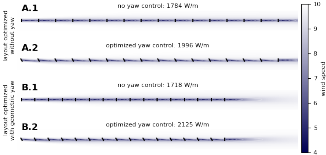
Figure 3. A simple one-dimensional optimization of a 16-turbine 16-turbine wind power plant comparing the performance of the layout optimized without yaw control and the layout optimized with geometric yaw. Figures 3A.1 and 3A.2 show the layout that was optimized assuming no yaw control. Figures 3B.1 and 3B.2 show the layout that was optimized using the geometric yaw relationship. Figures 3A.1 and 3B.1 show the plant and performance for each optimized layout without yaw control. Figures 3A.2 and 3B.2 show these same layouts, but with the final optimized yaw angles.
