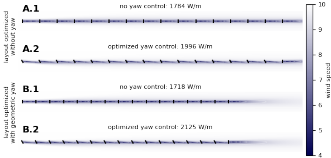
Figure 3. A simple one-dimensional optimization of a 16-turbine wind power plant comparing the performance of the layout optimized without yaw control and the layout optimized with geometric yaw. Figures 3A.1 and 3A.2 show the layout that was optimized assuming no yaw control. Figures 3B.1 and 3B.2 show the layout that was optimized using the geometric yaw relationship. Figures 3A.1 and 3B.1 show the plant and performance for each optimized layout without yaw control. Figures 3A.2 and 3B.2 show these same layouts, but with the final optimized yaw angles.
