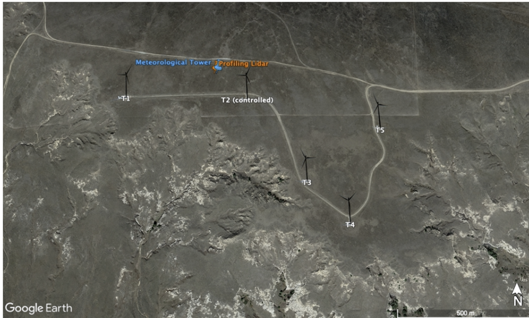
Figure 1. Site of the wake-steering field campaign, focusing on flow from the north through five turbines (T1–T5), with wake steering applied to T2 to benefit T3; inflow measurements come from a co-located meteorological tower and profiling lidar upstream. Maps data from Google, ©2023 CNES / Airbus, Maxar Technologies, USDA/FPAC/GEO
