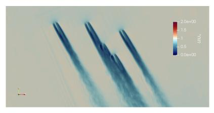
(a) S=6.5 m/s,  $D=332^\circ$  , TI=2% with  $\psi=0^\circ$  (08:08 UTC)
