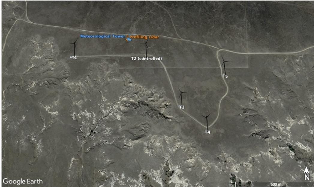
**Figure 1.** Site of the wake-steering field campaign, focusing on flow from the north through 5 turbines (T1–T5), with wake steering applied to T2 to benefit T3; inflow measurements come from a co-located meteorological tower and profiling lidar upstream. Maps data from Google, ©2023 CNES / Airbus, Maxar Technologies, USDA/FPAC/GEO
