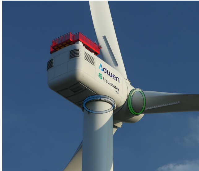
Figure 1. Wind turbine pitch bearing (green, also called blade bearing) and yaw bearing (blue). ©Fraunhofer IWES/Jens Meier
