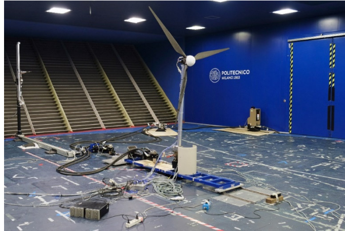
Figure 3: UNAFLOW Rotor during tests in the wind tunnel. Image courtesy of Politecnico di Milano.
