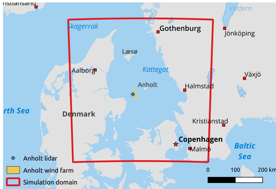
Figure 1. Map of the simulation domain. On every side of the domain 20 points are used for relaxation and spin up zones. These relaxation and spin up points are not used in the analysis. Made with Natural Earth.
