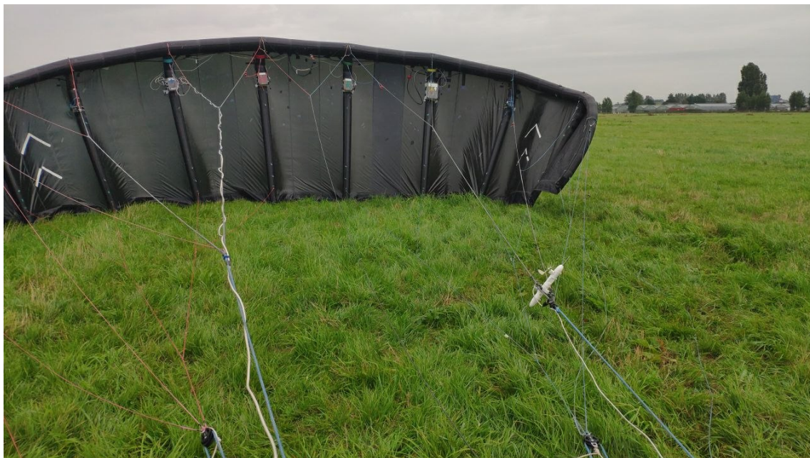
Figure 2. Fully instrumented V3.25B kite before launch (photo courtesy of Kitepower B.V.).
