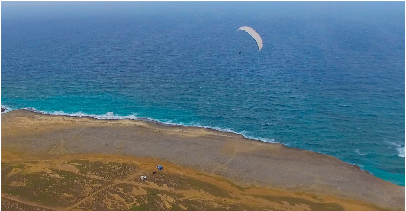
Figure 1. AWE system of Kitepower B.V. with a 60 m 2 kite and ground station integrated in a standard 20 ft container in operation on the Caribbean island Aruba in October 2021 (photo courtesy of Kitepower B.V.).
