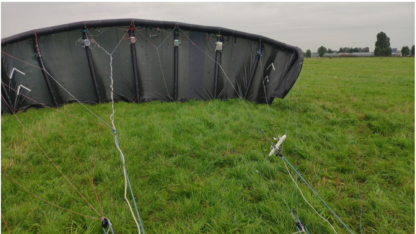
Figure 2. Fully instrumented V3.25B kite before launch (photo courtesy of Kitepower B.V.).
