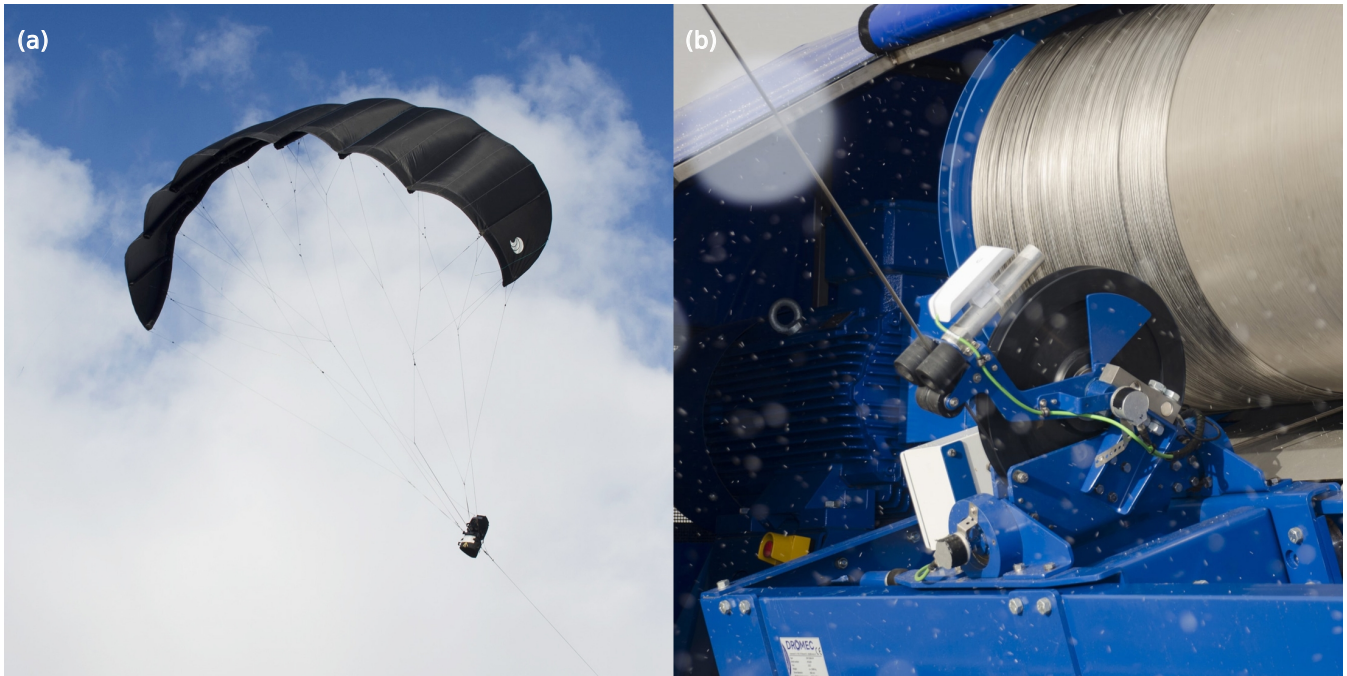
Figure 1. AWE system with (a) 25 m 2 V3.25B kite and (b) 100 kW ground station in operation in 2018 (photos courtesy of Kitepower B.V.).
