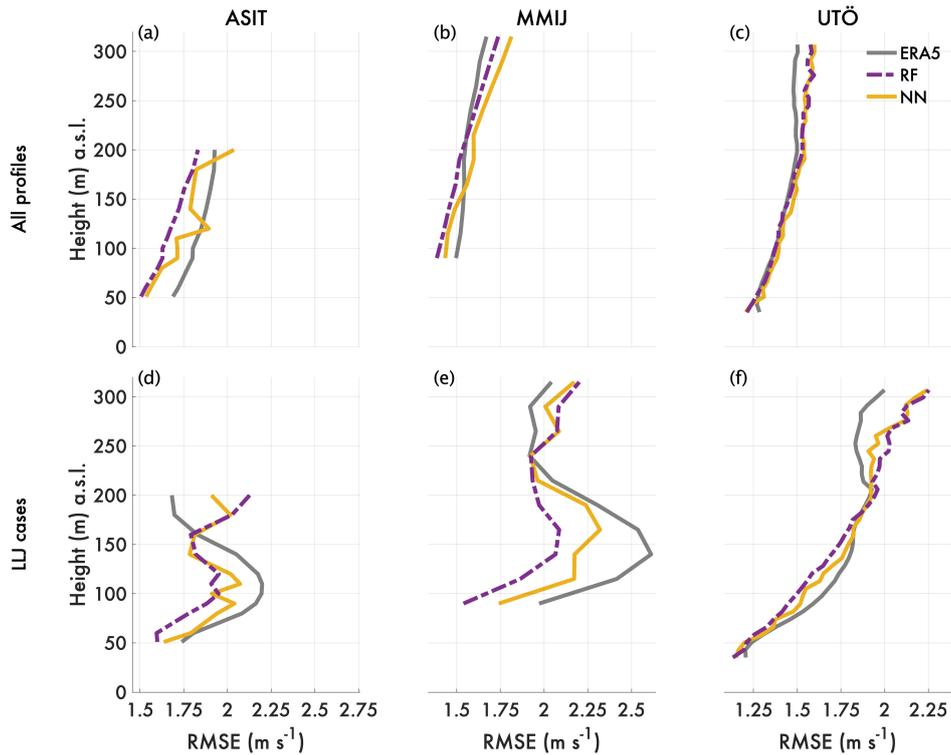
**Figure 6.** (a–c) RMSE for wind speed profiles for ERA5 (gray), the RF (purple), and the NN (yellow) for ASIT, MMIJ, and Utö. The values of RMSE are calculated relative to the lidar observations and the results are valid for the test period. Panels (d–f), present RMSE for ERA5 and the ML models for the subset of the test data with LLJs (crit. 1) in the lidar profiles.
