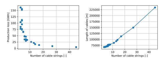
**Figure 5.** Number of cable strings as a function of the cable length (left) and Annual electrical losses as a function of the number of cable strings (right)
