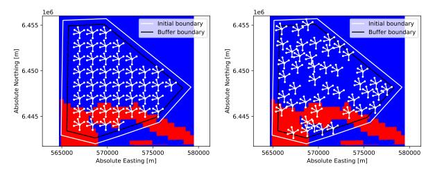
Figure 9. Grid-based layout (left) and optimized layout (right) showing WTGs with their mooring lines on the binarized bedrock map for Broadshore site
