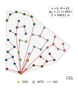
Figure 3. Optimized cable routing with one OSS and a max of 6 FOWT per cable string
