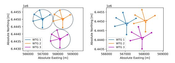
**Figure 1.** Possible layouts for three turbines using the circular constraint where the mooring lines are constrained in circles (left) and geometrical constraint where the mooring lines can be overlapping (right)
