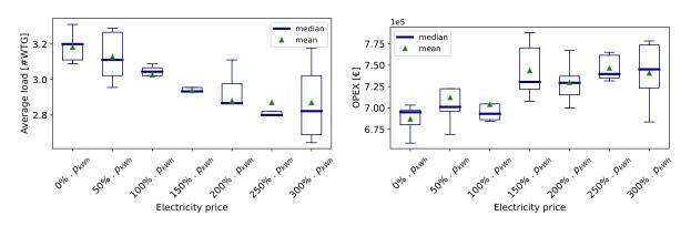
Figure B2. Results of the sensitivity analysis on the electricity price - Average load and OPEX
