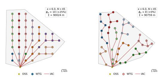
Figure 8. Grid-based layout (left) and optimized layout (right) and their associated optimized cable routings for Broadshore site
