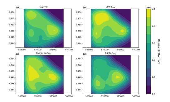
**Figure B14.** Density heat-maps of FOWT positions, for different unit cable cost levels *x-axis: Absolute Easting [m]*, *y-axis: Absolute Northing [m]*
