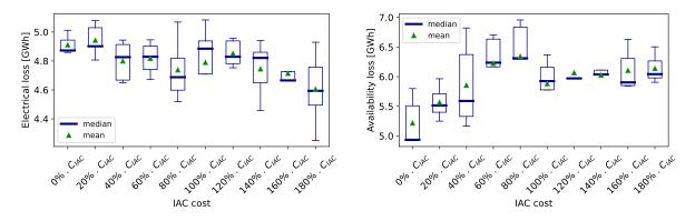
Figure B12. Results of the sensitivity analysis on the unit cable cost - Electrical and availability losses
