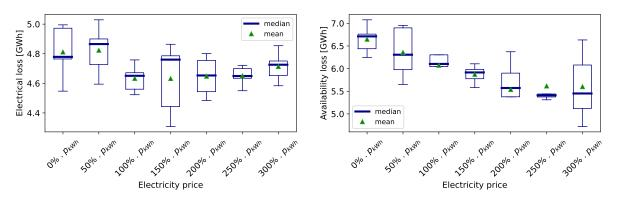
Figure 12. Results of the sensitivity analysis on the electricity price - Electrical and availability loss
