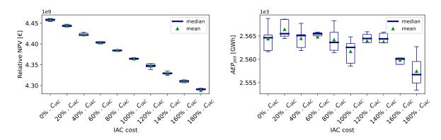
Figure B9. Results of the sensitivity analysis on the unit cable cost - relative NPV and potential AEP
