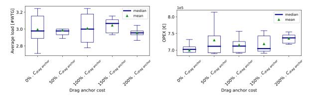
Figure B7. Results of the sensitivity analysis on the anchors cost - Average load and OPEX
