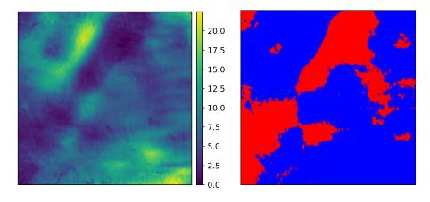
Figure 2. Non-binarized (left) and binarized (right) maps of the bedrock depth under the seafloor
