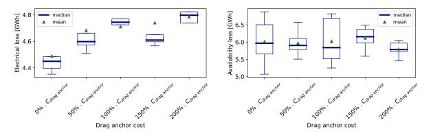
Figure B6. Results of the sensitivity analysis on the anchors cost - Electrical and availability losses
