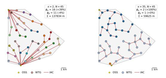
**Figure 6.** Cable routing for  $\kappa = 2$  (left) and  $\kappa = 35$  (right)
