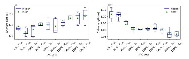
Figure B10. Results of the sensitivity analysis on the unit cable cost - Anchors costs and cable length
