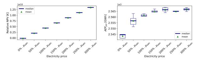
Figure 10. Results of the sensitivity analysis on the electricity price - relative NPV and potential AEP
