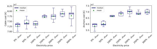
Figure 11. Results of the sensitivity analysis on the electricity price - CAPEX components (cable cost and anchors cost)
