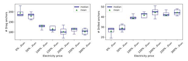
Figure B1. Results of the sensitivity analysis on the electricity price - Number of drag and drilled anchors
