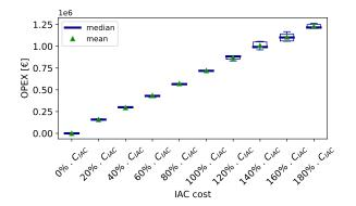
Figure B13. Results of the sensitivity analysis on the unit cable cost - OPEX
