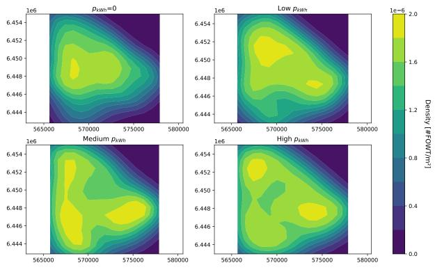
Figure 13. Density heat-maps of FOWT positions, for different electricity price levels *x-axis: Absolute Easting [m]*, *y-axis: Absolute Northing [m]*
