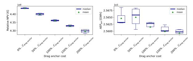
Figure B3. Results of the sensitivity analysis on the anchors cost - relative NPV and potential AEP
