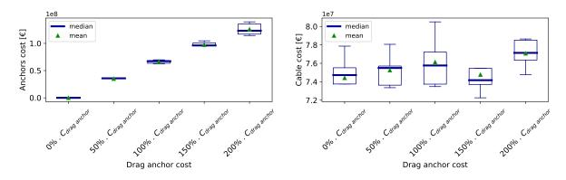
Figure B4. Results of the sensitivity analysis on the anchors cost - Anchors costs and cable cost
