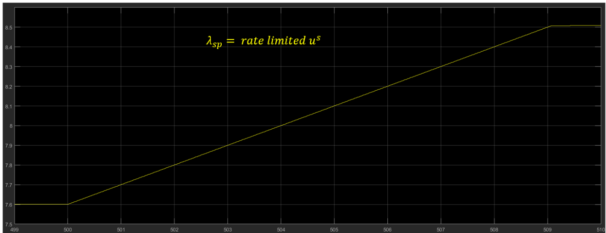
Figure B: Simulink Scope showing TSR command to the ROSCO controller – Eroded blade ( U=8\text{m/s} , TI = 10\% ).
