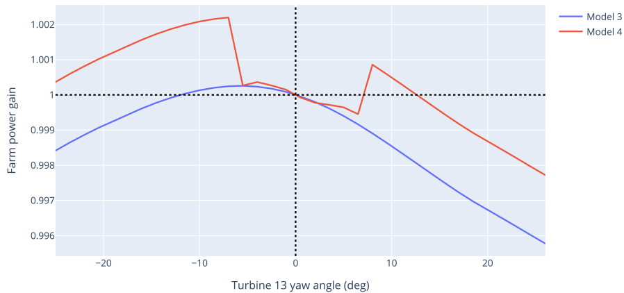
Figure 19. Predictions of farm power gain as a function of turbine 13’s yaw angle with and without the output corrector (Model 4 and 3, respectively). For model 4, the full output corrector is used for yaw error values between -6 and +7 degrees. Outside of this range, all individual models in the ensemble will revert back to the engineering wake model, if that model depends on turbine 13’s yaw error. All other models in the output corrector ensemble are used for the entire range.
