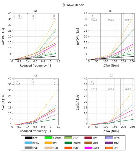
Figure 16 Amplitude of normalized wake deficit oscillations as a function of reduced frequency and rotor thrust for surge (a, b) and pitch cases (c, d). Dashed lines represent the FVW results and solid lines represent either the CFD or experimental results.
