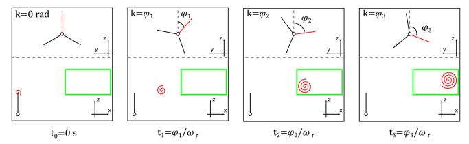
Figure 3 Sketch of the definition of vortex age. The time that passes from the formation of the tip vortex to the time it is analyzed is expressed in terms of the azimuth angle of the blade.
