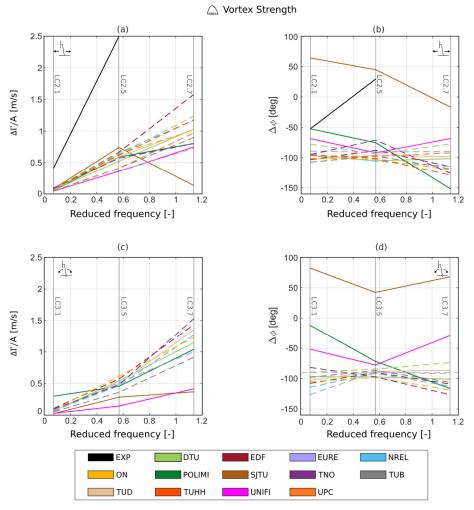
Figure 12 Amplitude and phase shift of tip vortex strength for surge (a, b) and pitch (c, d) cases. Dashed lines represent the FVW results and solid lines represent either the CFD or experimental results.
