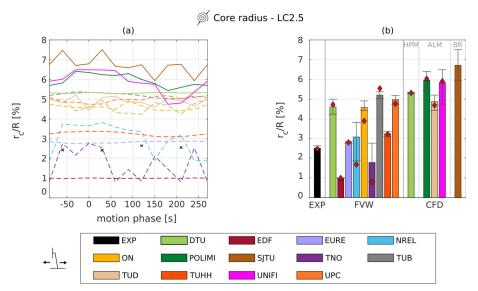
Figure 10 (a) Tip vortex core radius during platform motion. Dashed lines represent the FVW results, solid lines represent the CFD results, and the black crosses represent the experimental data. (b) Average core radius during surge motion. The whiskers represent the minimum and maximum values of the core radius during the cycle of motion, and the red diamonds indicate the fixed-bottom value.
