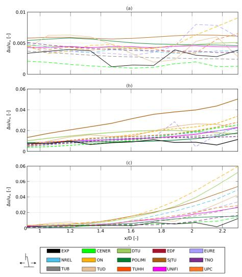
Figure 17 Amplitude of streamwise velocity oscillations at the frequency of platform motion calculated from each of the along-wind probes as a function of rotor distance for the analyzed surge cases. (a) LC2.1: A = 0.125 m,  $f_r = 0.071$ , (b) LC2.5: A = 0.035 m,  $f_r = 0.568$ , (c) LC2.7: A = 0.008 m,  $f_r = 1.137$ . Dashed lines represent the FVW results and solid lines represent either the CFD or experimental results.
