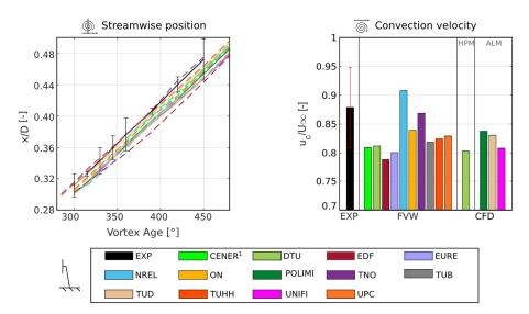
Figure 6 Tip vortex streamwise position (left) and convection velocity (right). Dashed lines represent the FVW results and solid lines represent either the CFD or experimental results. <sup>1</sup>Error bars represent the standard deviation of the experimental data.
