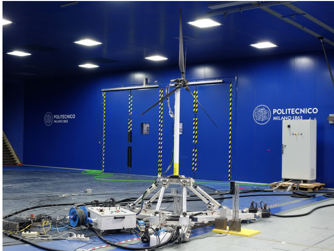
Figure 1. Experimental setup in the Polimi wind tunnel. “CS1” and “CS2” are respectively the coordinate systems for platform motion and rotor forces.
