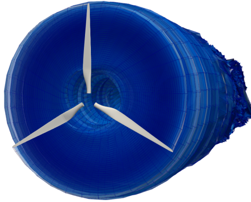
Figure 2. Panel method simulation results of the UNAFLOW rotor and its wake.
