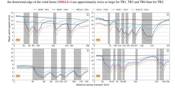
Figure 9. Transects of the mean wind speed at turbine hub height for the different wind farm scenarios. These transects correspond to the four lines in Fig. 1. Wind data is only considered when the wind direction deviates within  $+-15\pm15^{\circ}$  from the transect orientation (W to E) at the middle grid cell of each transect. Grey shadings represent wind farmsfarm locations.
