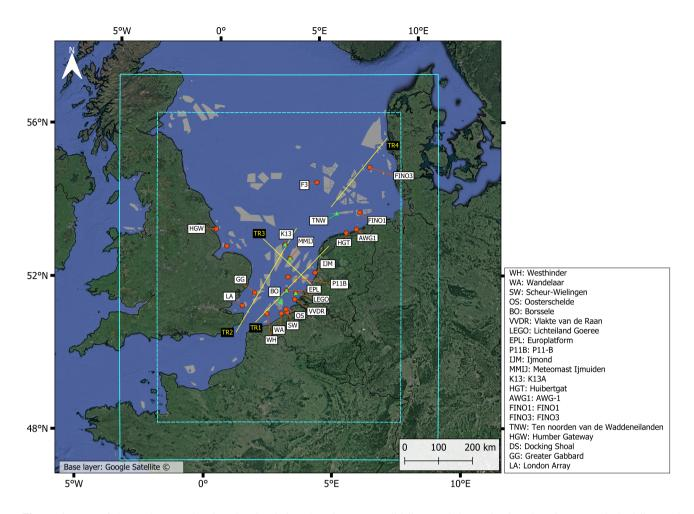
**Figure 1.** Map of the study area showing the simulation domain (cyan, solid line) and the evaluation domain (cyan, dashed line). Also the locations of the in situ measurement stations (orange dots) and lidar stations (green triangles) that are used for the model evaluation are indicated, in addition to the hypothetical future wind farm layout (grey polygons) and the four analysis transects TR1-TR4 TR1-TR4 (yellow lines) used for the wind farm simulations. Map created Created using QGIS3.4.
