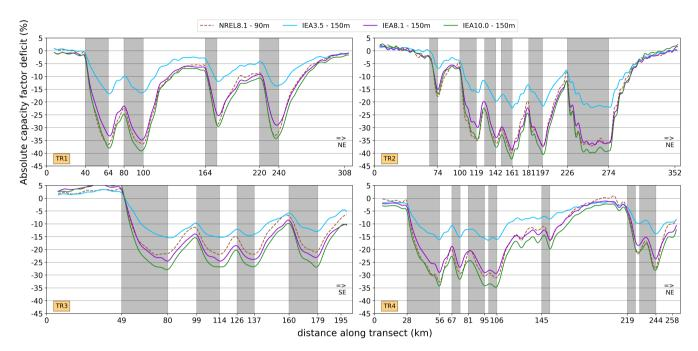
Figure 10. Transects of the absolute capacity factor deficit at hub height for the different wind farm scenarios. These transects correspond to the four lines in Fig. 1. Wind data is only considered when the wind direction deviates within  $+15\pm15^{\circ}$  from the transect orientation (W to E) at the middle grid cell of each transect. Grey shadings represent wind farmsfarm locations.
