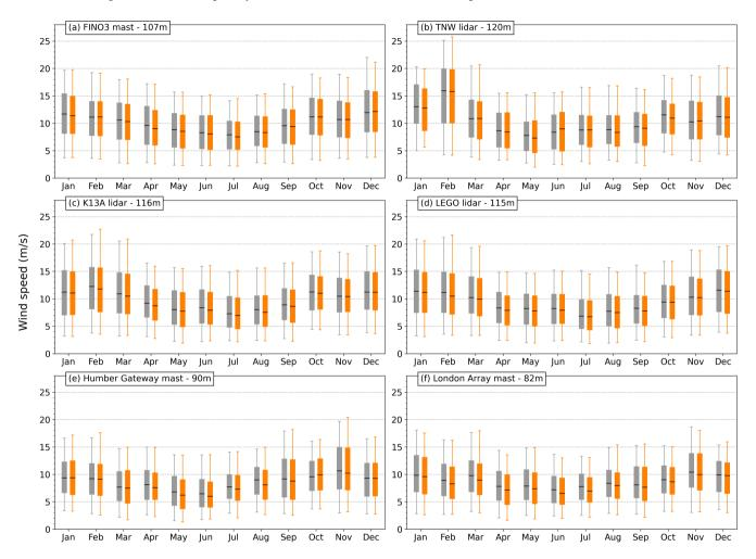
**Figure 5.** Boxplots representing the multi-year wind speed distribution per month for the observations (grey) and the model (orange). Shown for the three masts and three lidar stations at turbine hub height. The box corresponds to the Q25-Q50-Q75 wind speeds. The lower and upper whisker are the Q5 and the Q95 percentiles, respectively.
