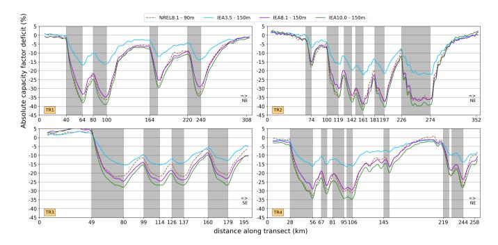
Figure 10. Transects of the absolute capacity factor deficit at hub height for the different wind farm scenarios. These transects correspond to the four lines in Fig. 1. Wind data is only considered when the wind direction deviates within  $\pm 15^{\circ}$  from the transect orientation (W to E) at the middle grid cell of each transect. Grey shadings represent wind farm locations.
