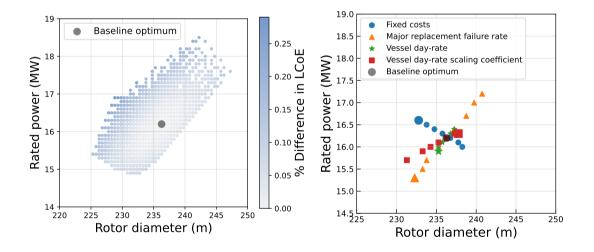
**Figure 10.** (a) Sensitivity of the optimum design to O&M model parameters for random combinations of parameter values. (b) One-at-the-time variation per parameter (the larger markers correspond to the lower end of the parameter variation range).
