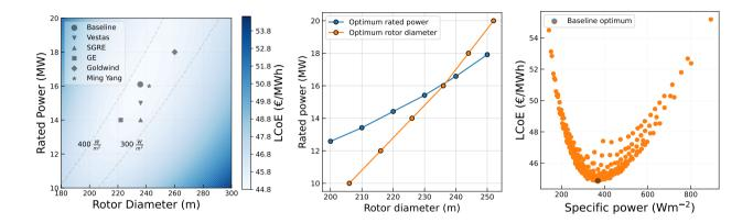
**Figure 7.** (a) Response map of LCoE w.r.t. the two design variables. (b) Optimum rated power and rotor diameter per constrained diameter and rated power, respectively. (c) LCoE plotted against the specific power
