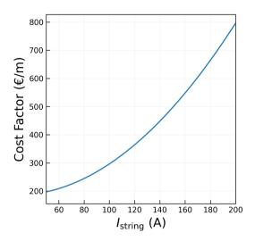
Figure 1. Infield cable cost as a function of total current in a string
