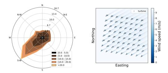
Figure 3. (a) Directional wind speeds and probabilities for the hypothetical site. (b) Farm layout for a 15 MW turbine and 1 GW of farm power.
