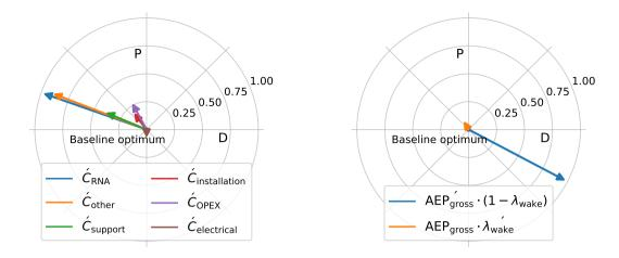
Figure 8. Cost and AEP gradient components at the optimum for the baseline case.
