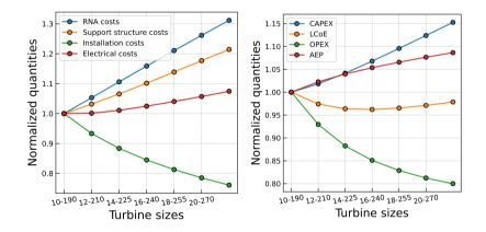
**Figure 5.** (a) Change in components of capital expenditures (normalized) w.r.t. upscaling of turbines with the same specific power. (b) Change in crucial farm-level quantities (normalized) w.r.t. upscaling of turbines with the same specific power.
