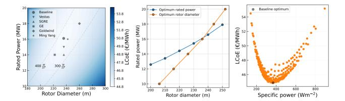
**Figure 7.** (a) Response map of LCoE w.r.t. the two design variables. (b) Optimum rated power and rotor diameter per constrained diameter and rated power, respectively. (c) LCoE plotted against the specific power
