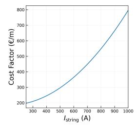
Figure A1. Infield cable cost as a function of total current in a string
