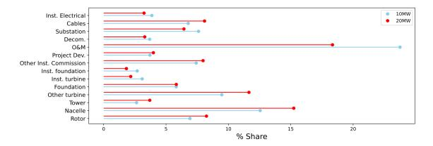
Figure 4. LCoE cost breakdown of a 10 MW turbine and a 20 MW turbine, both with a specific power of 350 Wm<sup>-2</sup>.
