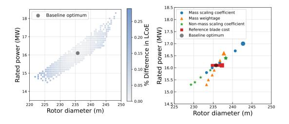
**Figure 9.** (a) Sensitivity of the optimum design to rotor model parameters for random combinations of parameter values. (b) One-at-the-time variation per parameter (the larger markers correspond to the lower end of the parameter variation range).
