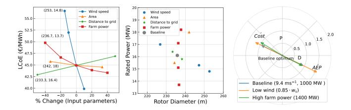
**Figure 11.** (a) Change in LCoE w.r.t. change in design conditions. (b) Change in the optimum w.r.t. change in design conditions. (c) Change in gradients at the baseline optimum for different design conditions.
