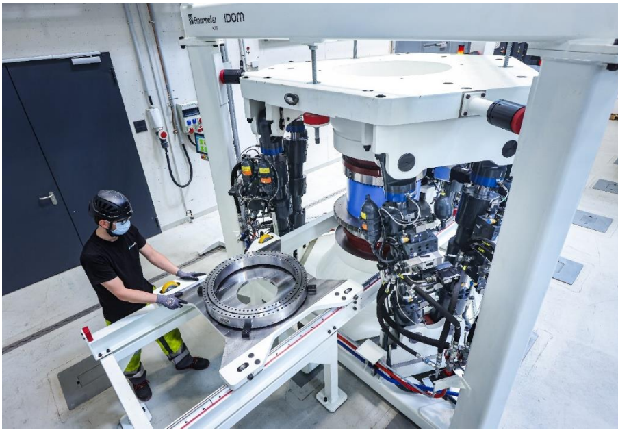
325 Figure 13: BEAT1.1 test rig and downscaled blade bearing 13229 (©Fraunhofer IWES/ Ulrich Perrey)
