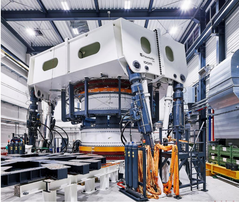
365 Figure 15: BEAT6.1 test rig (©Fraunhofer IWES/ Marcus Heine)
