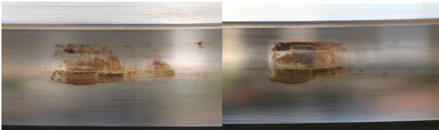
Figure 18: Severe wear marks on the raceway of 4pBB 51818
