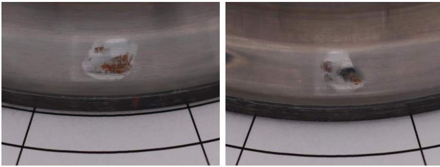
Figure 17: Wear marks on the type 7220 bearings
