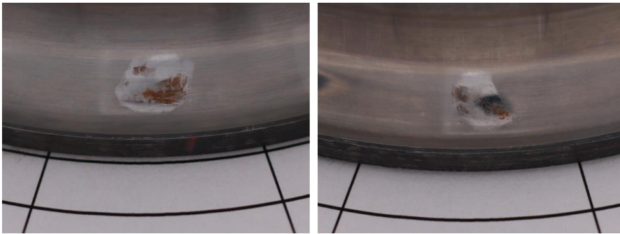
Figure 17: Wear marks on the type 7220 bearings
