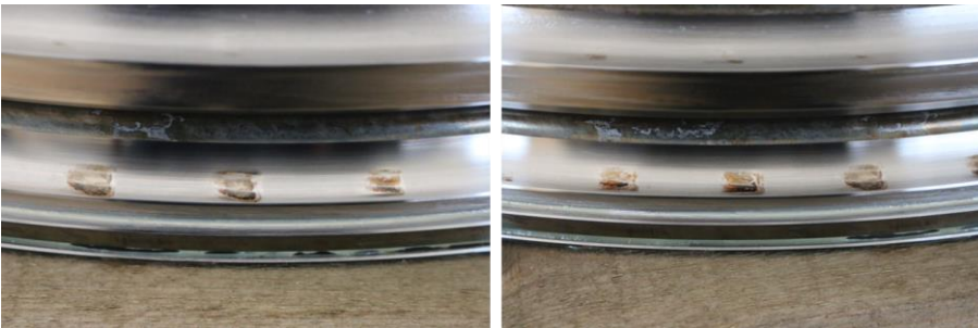
445 Figure 21: Wear marks on the raceways of the downscaled blade bearings 13229 lubricated with grease no.2
