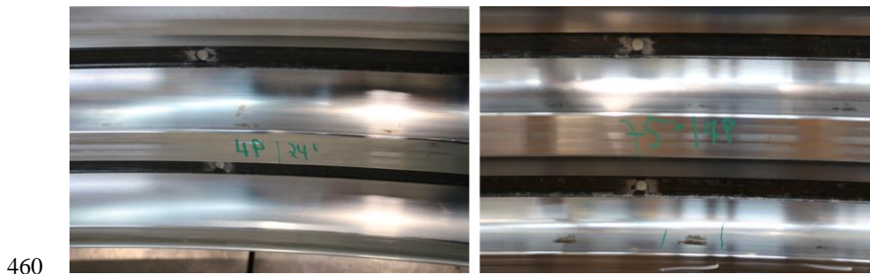
460 Figure 22: Wear marks on the raceways of the type 12480 blade bearing outer ring
