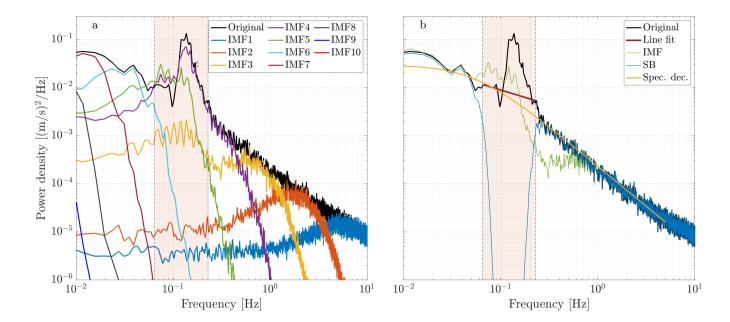
Figure D1. (a) Power spectra of the vertical velocity fluctuation w' (illustrated in Fig. 6d) and its decomposed IMFs (for n=10); and (b) comparison of different wave-turbulence decomposition methods: stopband technique (blue curve), spectral linear transformation (red line), the EMD method after removing IMF4 (green curve), and the spectral decomposition method proposed in this paper (yellow curve). The colored areas in this figure show the selected wave frequency band.
