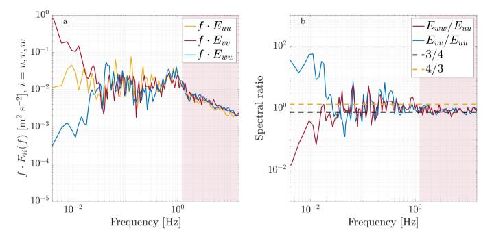
Figure B1. (a) Three-dimensional velocity spectra  $f \cdot E_{ii}(f)$  for i = u, v, and w showing the spectral regions of the wave-affected peaks and the inertial subrange; and (b) velocity spectra ratios with horizontal dashed yellow and black lines indicating the value of 4/3 and 3/4, respectively.
