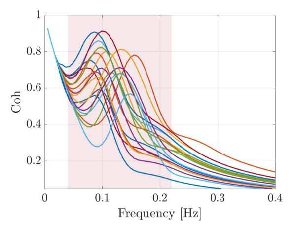
Figure C1. Theoretical coherences are generated based on the fundamental parameters listed in Table C1. To create 20 ensembles, I perturb  $H_s$  within the range of [0.5, 1.5],  $T_p$  within [5, 12],  $A_1$  within [0.1, .5], and  $A_2$  within [0.02, 0.1]. It is important to note that in the theoretical model defined in Eq. (8), we only use Term1 and Term2 to produce this figure.
