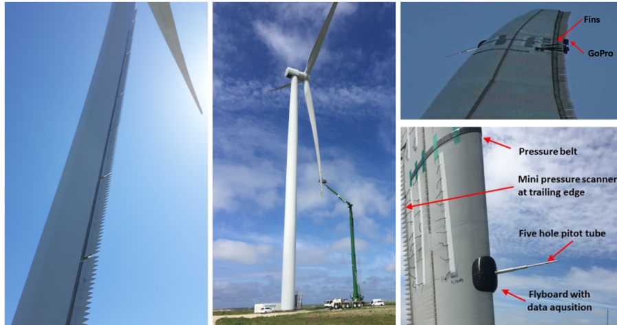
Figure 1. Left photo: Active flap placed on the trailing edge of the blade of the SWT-DD-120 turbine Prototype at the Høvsøre test field. Central photo: Installation of the flyboard and pressure belt in June 2020. Bottom right photo: Close look at the flyboard and the pressure belt. Top right photo: Camera and fins installed to measure the flap deflection. Photos courtesy of SGRE and DTU.
