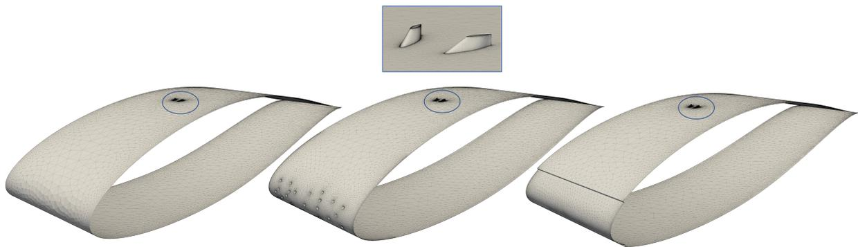
**Figure 13.** Mesh for rough (left), type 1 eroded (middle) and type 2 eroded (right) cases with CENER's Low Drag VGs.
