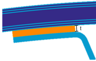
Figure 7. Close up of blade cross-section highlighting web-to-skin bondline thickness.
