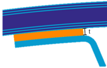
Figure 8. Close up of blade cross-section highlighting web-to-skin bondline thickness.
