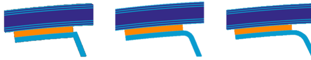
Figure 9. Cross-section detail showing range of corner radii from zero (left) through baseline (middle) to 50% larger (right).
