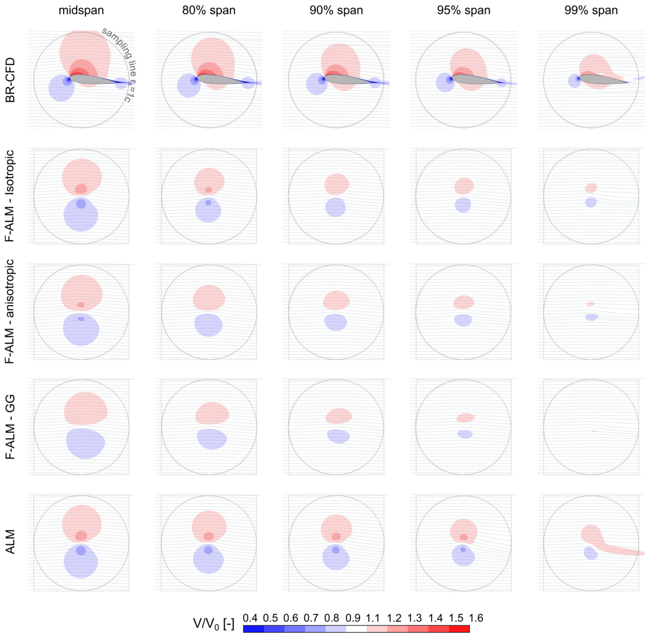
Figure 12 Comparison in terms of non-dimensional velocity magnitude V/V_0 between BR-CFD, Frozen ALM (F-ALM) and standard ALM (ALM) at different spanwise sections, for pitch=6^\circ .
